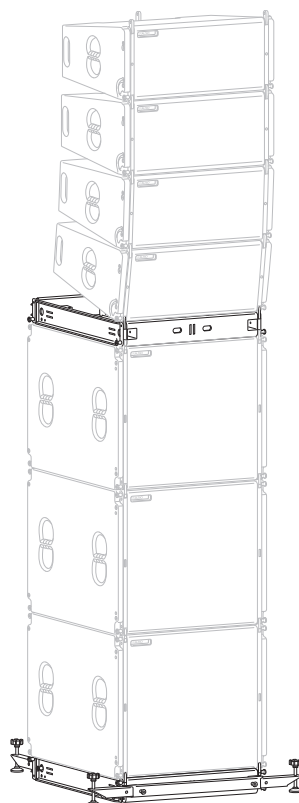
Figure 4.5 - System suggestion for a groundstack
